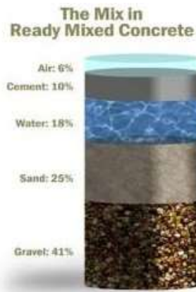
Figure 3.5.2. Typical composition of hydraulic cement concrete.
