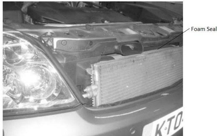
Location of Condenser
