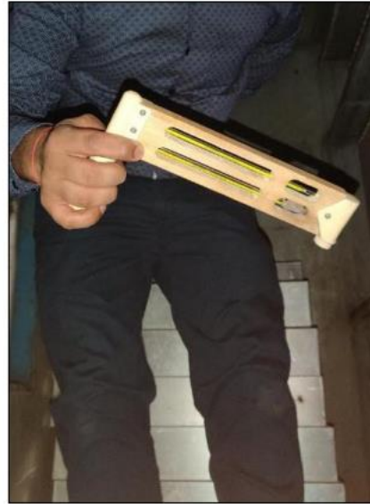
Pic no -15 Return air temperature with psychrometer
