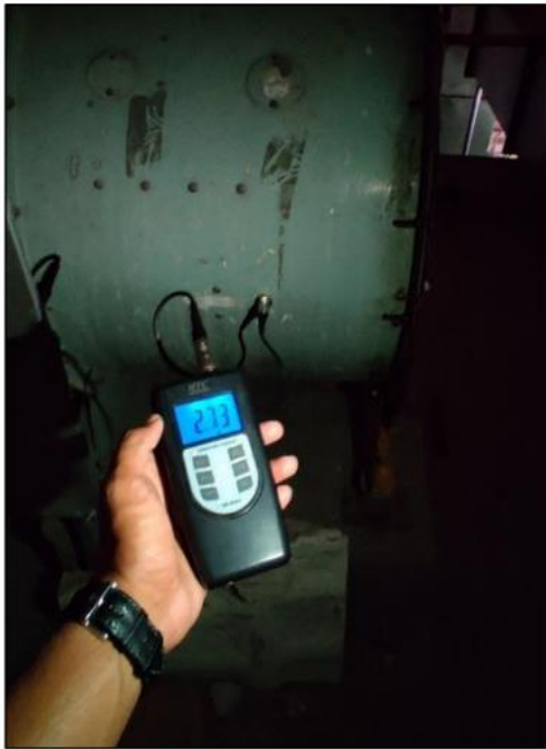
Pic no 20-Vibration measurement
