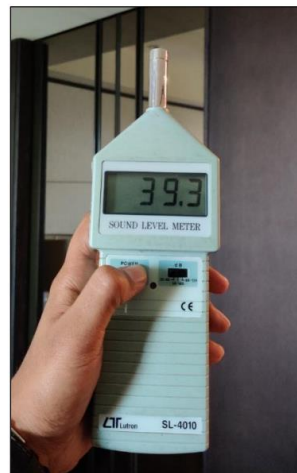
Pic 19- Sound level measurement
